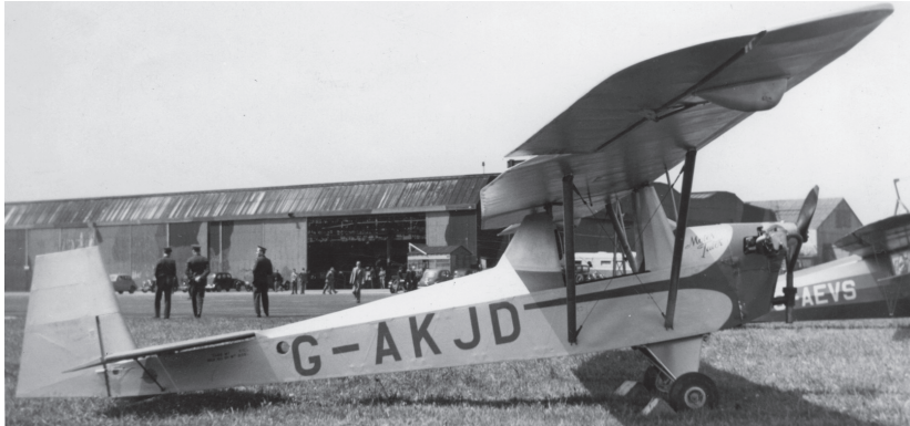
Left: The Motor Tutor G-AKJD, with 30hp JAP engine, which JM flew at Lasham in 1964, reporting a 50 mph cruise and 25 mph stall speed. He said later that it was the easiest aircraft to fly that he had ever tried, but it was written off in a crash at Dunstable the following month. (via JM Collection)
