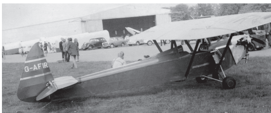
Below: Luton Minor G-AFIR was flown at Lasham in 1963. Second of the type, it was the first with parallel underwing struts. (Jack Meaden)
